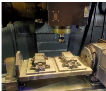
Gambar 2. Proses pengerjaan benda uji di CNC Milling Vertical Machining Centre Welle AA1165 BT40
