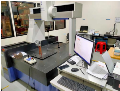
Gambar 6. Coordinate Measuring Machine (CMM) Mitutoyo Type 9106
